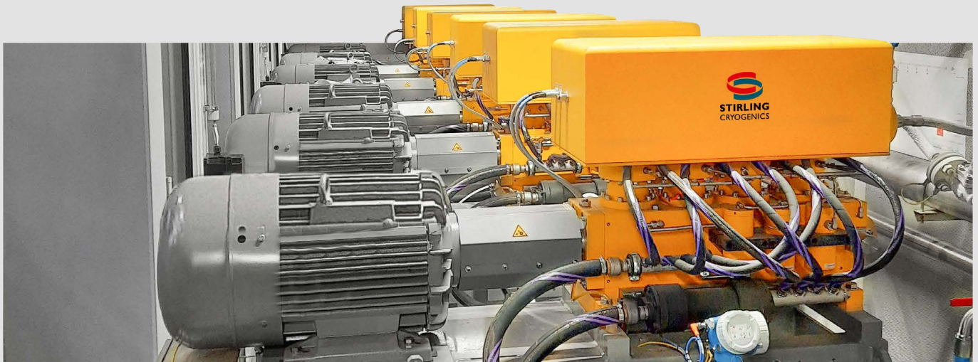
Containerized liquefaction system
