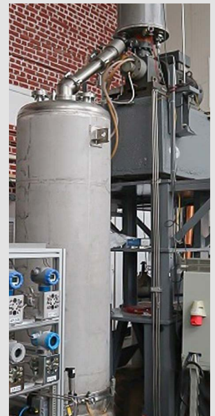
1973 Stirling Cryogenics Hydrogen Re-liquefier, photo courtesy ICSI, Romania
