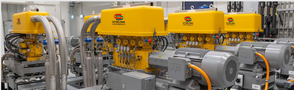
2019 Stirling Cryogenics Hydrogen Re-liquefier for Cold Neutron Source at RID, photo courtesy Reactor Institute Delft, The Netherlands
