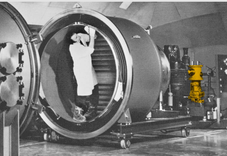
Two-stage Stirling Cryogenerator type SPC-1T; cooling shielding of a vacuum chamber at both 80 and 20 K temperature level (1960's)
