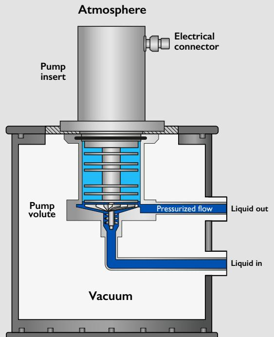
The design of the Stirling Cryogenics liquid gas pumps also allows them to be used as a gas circulator. When they are used as a circulator, the motor is set at a higher velocity to achieve sufficient gas flow. This feature is utilized during the cooling down phase of a system. Instead of pumping cold liquid into the application, causing thermal shock, cold gas is circulated to cool down the application gradually reduce temperature.
