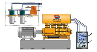
To circulate the helium, the Stirling SPC-4T Cryogenerator is equipped with integrated CryoFans (cryogenic circulators) in the vacuum space of the cold head. In many cases this eliminates the need for a separate cryostat. The CryoFans are selected based on the heat load, flow and dP of the customer's system.
