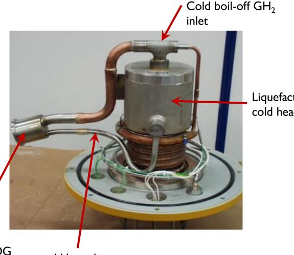
Two phase  $LH_2$  / BOG connection to  $LH_2$  vessel
